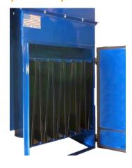
Carbon filter cell is used in cases where odors, gases, and vapors are associated with a process. Filter trays are removable and refillable. Activated carbon may be replaced with potassium permanganate. Available on models 1500 CFM and above.
